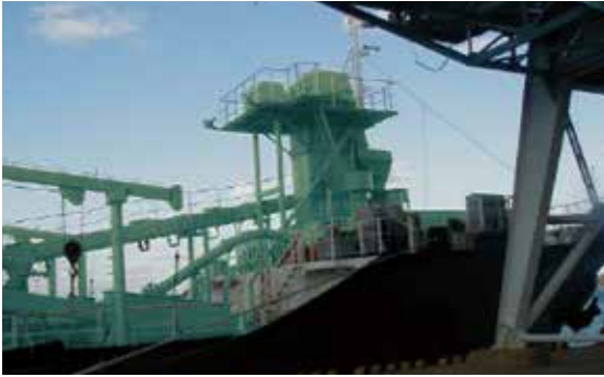
FA Series being used on a cement tanker and for conveying fly ash.
